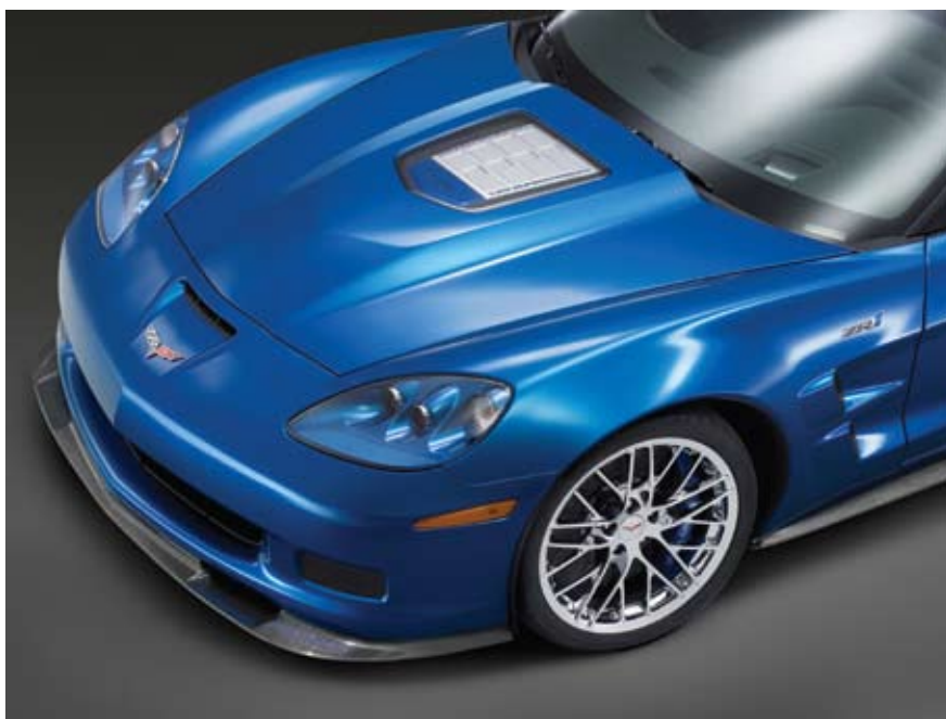
The 2009 Chevrolet Corvette uses carbon fiber on its exterior panels, including the hood and front splitter.
