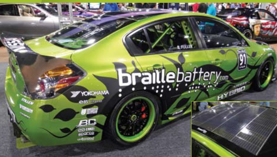
Braille Battery's "Hot Rod Hybrid" racecar is based on the Nissan Altima Hybrid. Features include a Braille carbon racing pack—Phase 1 Experimental, a 2.5-L I4 engine that runs on E85 fuel, a solar-panel charging system (inset), and Yokohama low-rolling-resistance high-performance tires.
