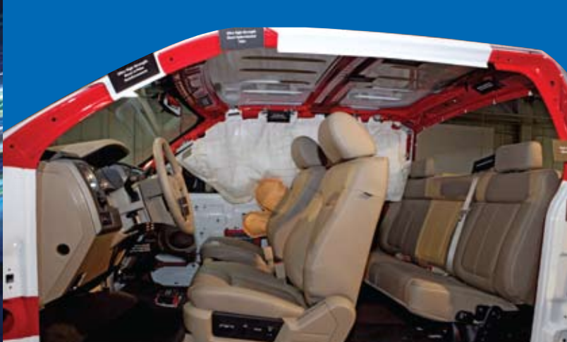
Ford's door aperture and double-walled rocker-panel insert are both stamped of high-strength steel to support the intrusion protection provided by boron steel door beams.
