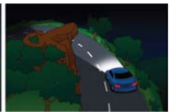
Approaching a curve with 3D map-guided headlights
