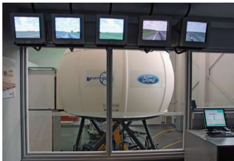
Ford's VIRTTEX module moves on six axes as drivers respond to simulated traffic experiences.
