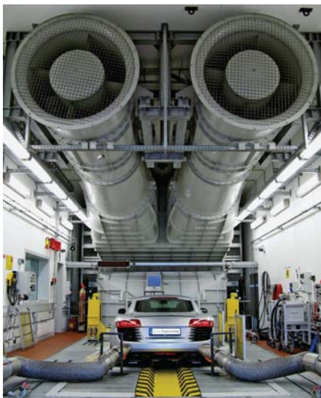
Among Bosch Engineering's testing capabilities is a 350-km/h (217-mph) dynamometer. The image shows Audi's R8 during testing.
