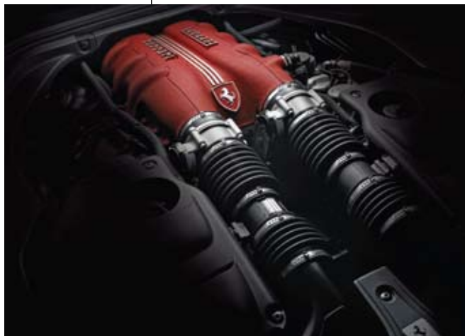
Heart of the matter: the California's 4.3-L naturally aspirated V8 engine gets direct injection—a Ferrari first.
