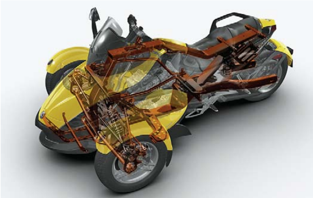
A Bosch Engineering vehicle dynamics software solution was developed for Bombardier Recreational Products' new three-wheeler, the Can-Am Spyder roadster. Its steel frame in surrounding spar technology has a low number of welds and high structural integrity. The frame's low weight and slender shape help to bring down the center of mass.
