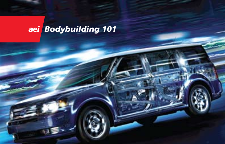
Ford relies on a hydroformed boron steel tube to reinforce the angular A-pillar-to-roof joint on the boxy Flex.
