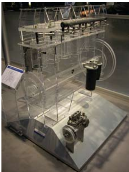
Delphi's new heavy-duty common-rail system, with engine-oil-lubricated cam and plunger pump, should be in production in 2012.
