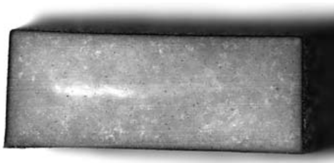
A Stanyl Diablo OCD2100 bar retains 90% of its original tensile strength after 2500 h of aging at continuous temperature levels up to 210°C (410°F).
